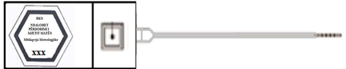
Fig.9. Plastic strap seal for measuring instruments prohibited for use by Metrological Supervision
