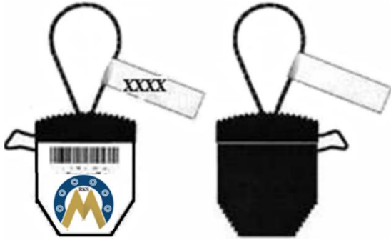
Fig. 8. The shape of plastic seal with verifying stamp
