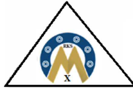
b. Verification stamp for measuring instruments that undergo only initial verification
